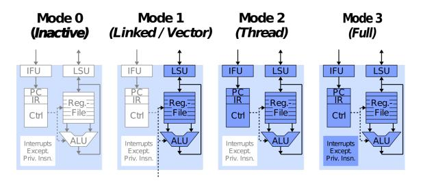
Figure 2.2.: ParaNut modes and required logic
