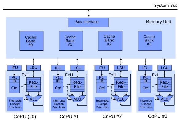
Figure 2.1.: A *ParaNut* instance with 4 cores
